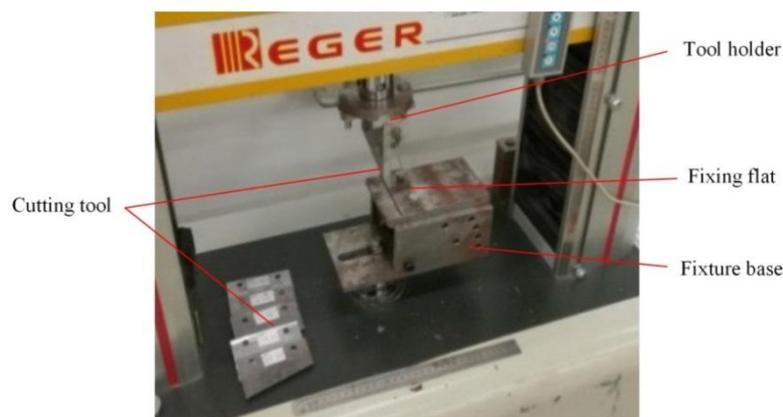
**Figure 1.** Shear device set up for the experiment.
