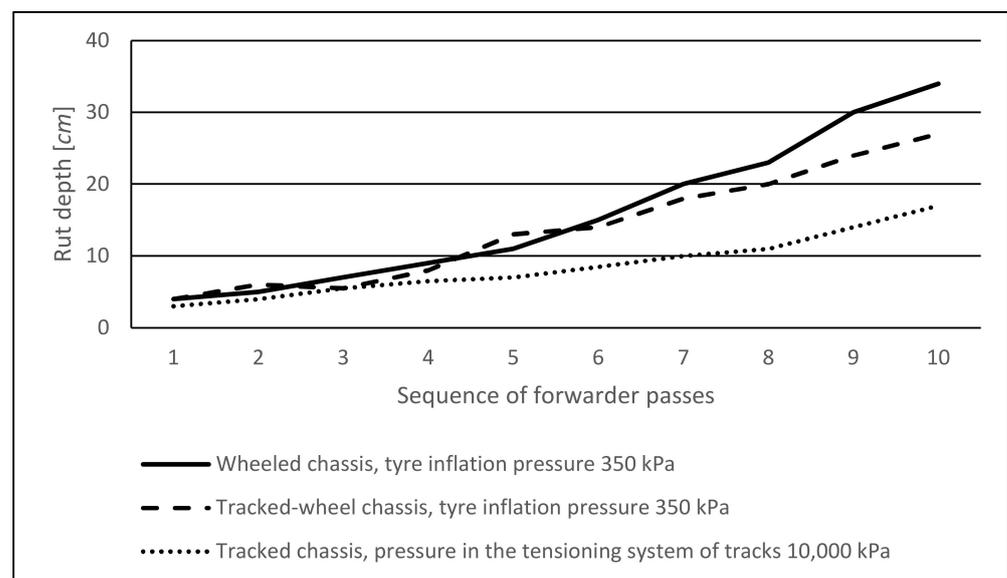
**Figure 10.** Driving track deepening in the soil profile after the pass of wheeled, tracked-wheel, and tracked type of the loaded forwarder.
