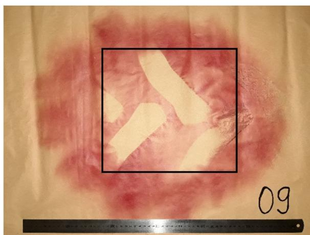
**Figure 2.** The outer boundaries of the tire tread imprint, front axle, tire inflation 250 kPa, load 0 kg.
