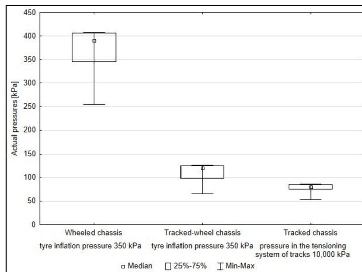
**Figure 6.** Range of values of induced actual pressures of rear axles in the respective forwarder chassis variants with the load during the first 10 passes.
