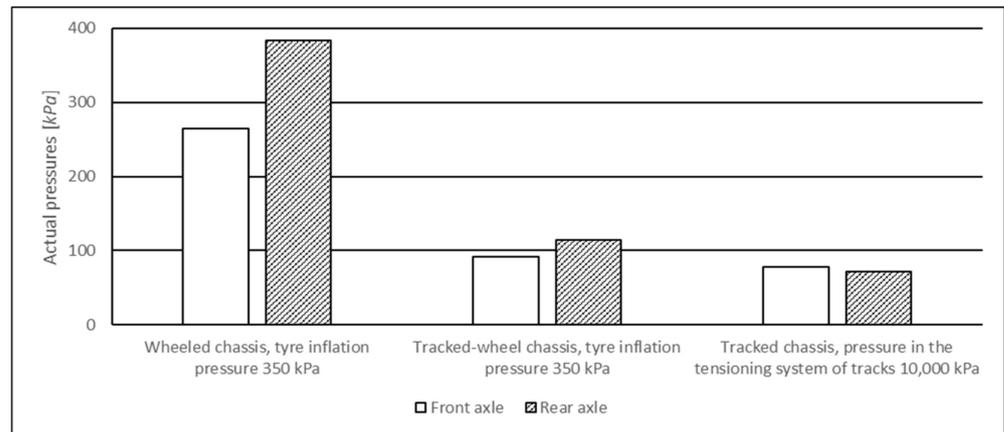
**Figure 5.** Average induced actual pressures in the respective chassis variants of the loaded forwarder.
