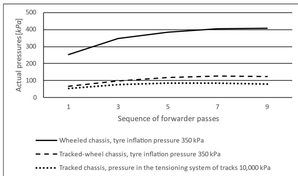
**Figure 7.** The course of induced actual pressures of rear axles in the respective forwarder chassis variants with the load during the first 10 passes.
