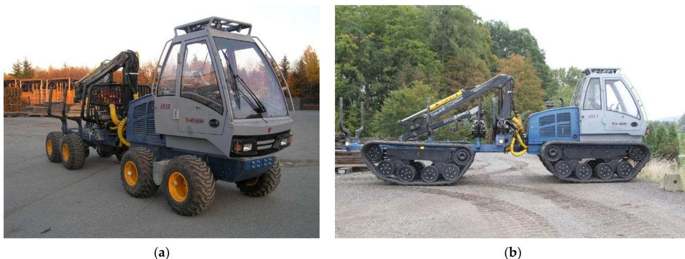
**Figure 1.** (a) Forwarder with the wheeled chassis; (b) forwarder with the tracked chassis.
