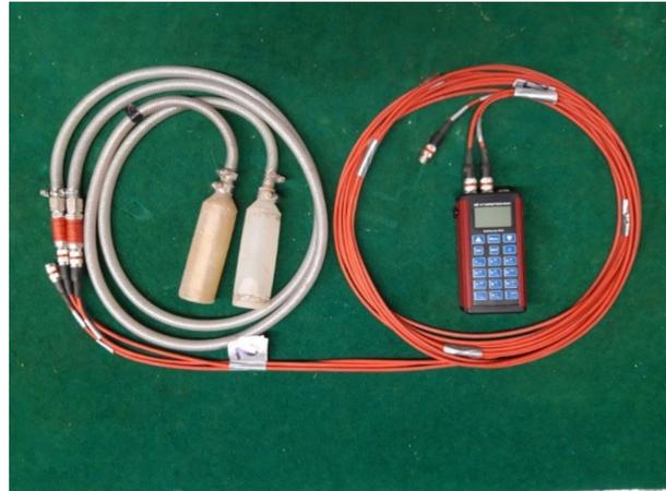
**Figure 3.** Measuring device for the determination of actual pressures in the soil profile during machine passes.
