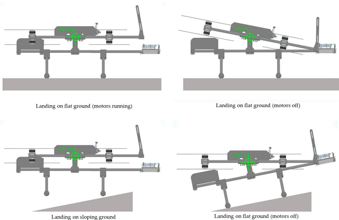
**Figure 10.** The battery, landing gear and hedge-trimmer sampling system were decoupled in the pitch axis from the flight controller and motors. The result was a highly responsive aircraft with the additional benefit of allowing landing on sloped sites. The prior version required flat ground, which was difficult to come by in the chosen test site.
