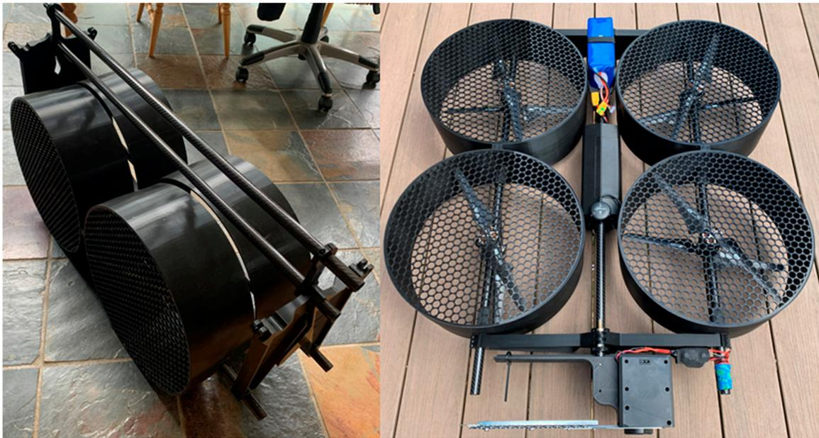
**Figure 7.** Version 3.0 protected the propellers with the use of 3D printed ducts. The design was capable of folding for ease of transport. The calculations used for estimating flight performance were found to be optimistic, with the system unable to fly out of ground effect.
