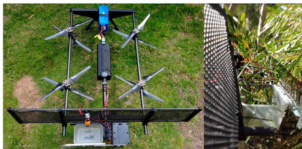
**Figure 8.** Version 3.1 of the canopy sampling UAS replaced the heavy, ducted fan system with a simple and lightweight, forward-facing shield to prevent collisions between the propellers and the canopy.
