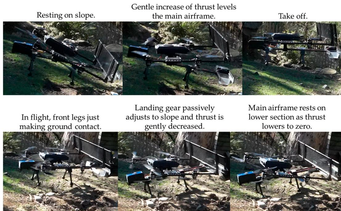
**Figure 11.** Real-world testing of the landing gear concept found it was highly effective on both upward and downward slopes, albeit unusual to pilot due to the large portion of the aircraft not responding directly to the control input.
