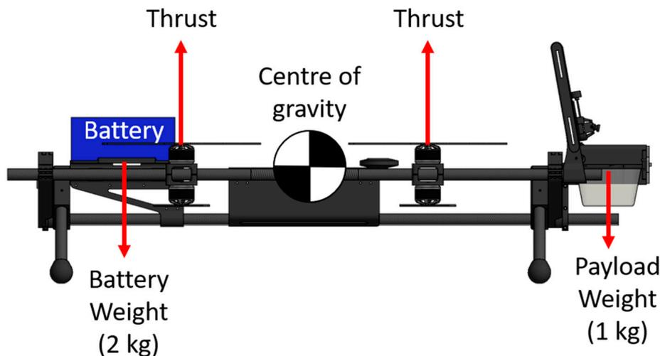
**Figure 1.** Our designs compensate for the offset payload mass by using the battery as a counterweight. With the battery weighing approximately 2 kg and the payload weighing approximately 1 kg, the payload can be further from the centre of mass than the battery, keeping the sampling operation as far in front of the propellers as practicable.
