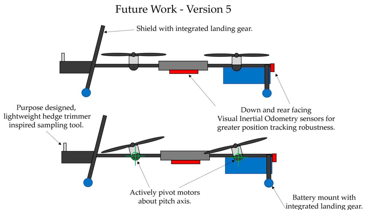
**Figure 14.** Our vision for the 5th iteration of this aircraft is inspired by Voliro [27], and would actively pivot the motor mounts about the pitch axis to separate forward and rearward movements from the pitch attitude of the entire airframe. This would likely be a better way to address the issues caused by the large moment of inertia about the pitch axis while also enabling take-off and landing on sloped terrain.
