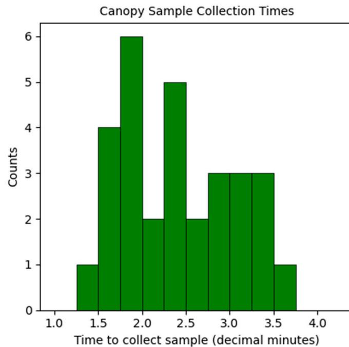
**Figure 12.** The distribution of the times taken to collect a canopy sample from arming to disarming the aircraft ( $n = 30$ ). An additional 5–10 min is required at the start and end of any sampling session to set up and pack away the equipment.
