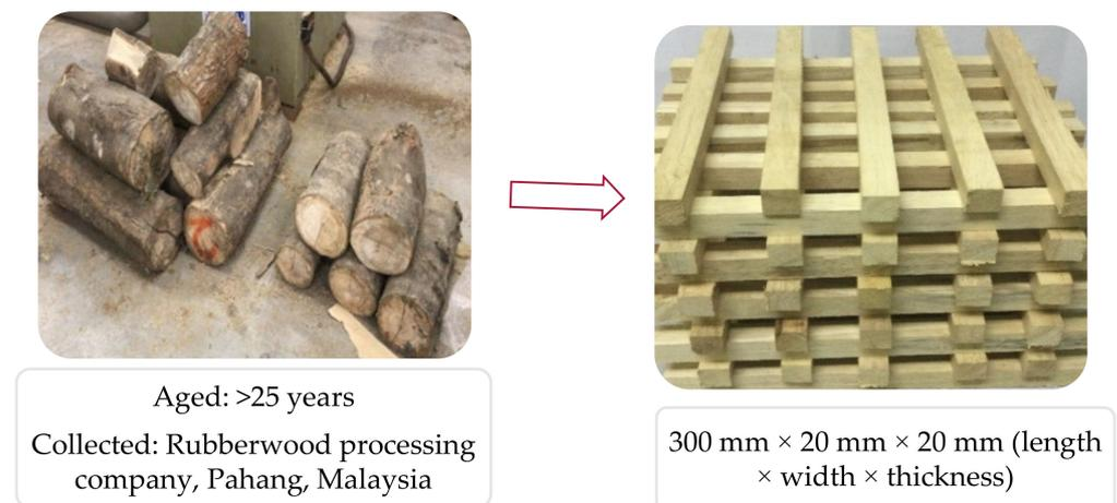
**Figure 1.** Photograph of prepared rubberwood samples with dimensions of 300 mm × 20 mm × 20 mm (length × width × thickness) for hydrothermal treatment.
