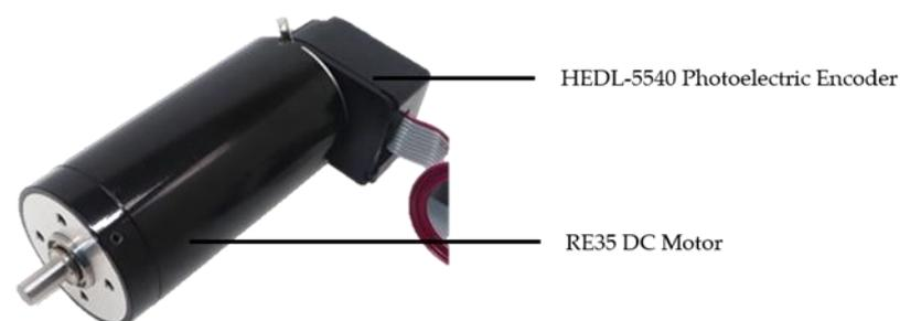
**Figure 4.** The RE35 DC motor with HEDL-5540 photoelectric encoder.
