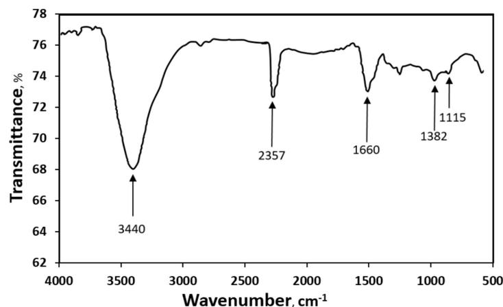
Figure 2. FTIR spectrum of MWCNTs.
