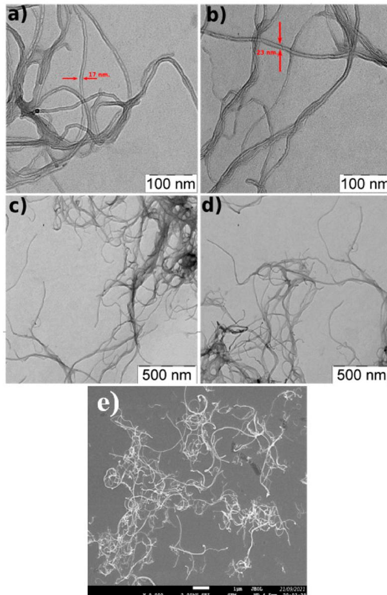
**Figure 3.** Image in MWCNT in TEM (a–d) and SEM (e).
