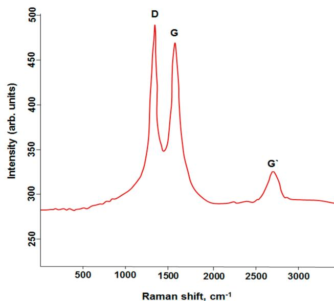
Figure 1. Raman spectrum of a MWCNT sample.
