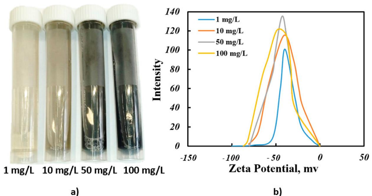
**Figure 4.** General view of colloidal solutions with different concentrations of MWCNTs (a) and the results of determining the zeta potential (b), certain concentrations of solutions.
