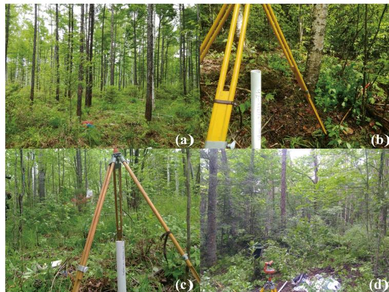
**Figure 2.** Sample plot photos. Figures (a–d) depict the site conditions of the actual study plots, with figures (b,c) specifically showing the standard plot corner stakes and the use of a compass clinometer for establishing the survey plot.
