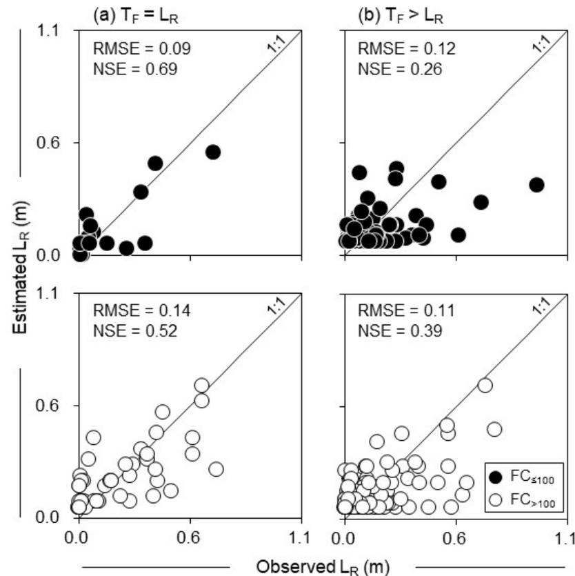
**Figure 6.** Relationship between the observed and estimated rising stream water level between  $\leq 100$  ha ( $FC_{\leq 100}$ ) and  $> 100$  ha ( $FC_{> 100}$ ) forested catchments during the two types of time of concentration, (a)  $T_F = L_R$  and (b)  $T_F > L_R$ .
