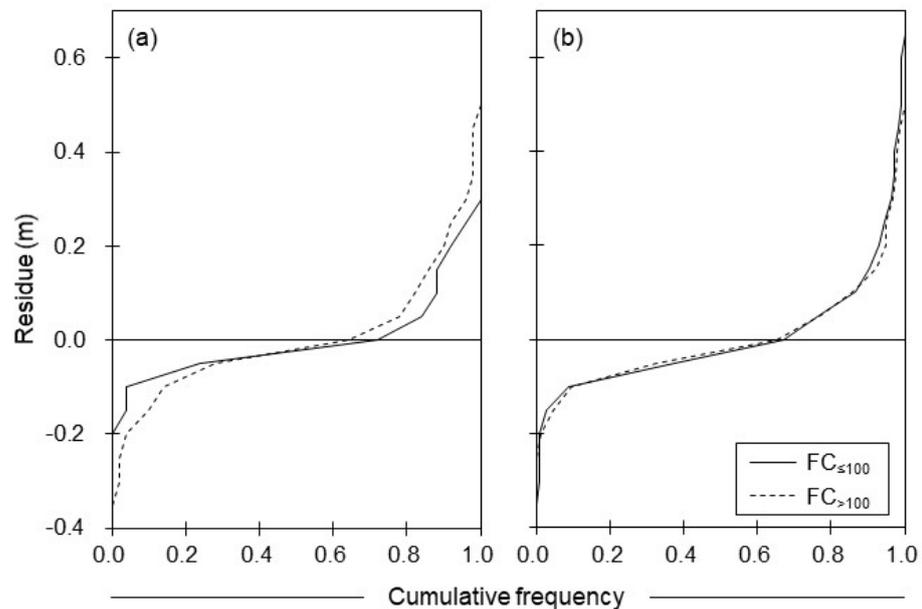
**Figure 7.** Cumulative frequency distributions for differences between observed and estimated rising water levels between  $\leq 100$  ha ( $FC_{\leq 100}$ ) and  $> 100$  ha ( $FC_{> 100}$ ) forested catchments in the two types of time of concentration, (a)  $T_F = L_R$  and (b)  $T_F > L_R$ .
