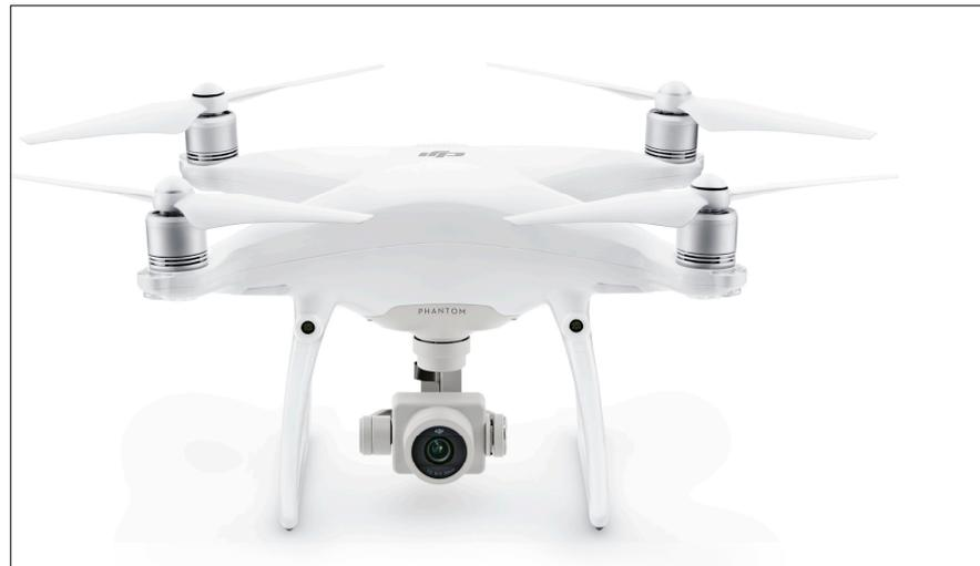
**Figure 2.** Unmanned aerial vehicle, model Phantom 4 Pro, used to acquire images.
