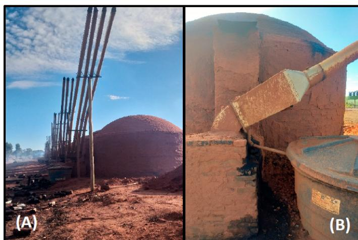
**Figure 1.** Carbonization liquids recovery devices (A); recovery apparatus basis (B).
