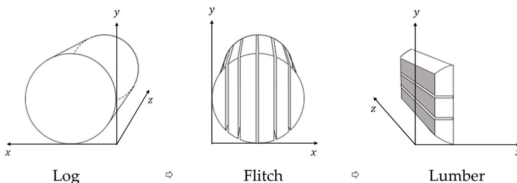
**Figure 1.** A two-step process for Log breakdown is commonly applied in sawmills in Korea. The  $x$ -axis and  $y$ -axis represent the width and height of the log's circular cross-section, respectively, while the  $z$ -axis represents the log's length.
