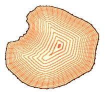
Figure 10. Discrete particles represent a cross-section of the wood.
