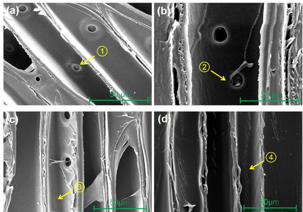
**Figure 2.** SEM images of tangential section at different incubation times. (a) the control sample, ① pit aspiration; (b) 4-week inoculated sample with *T. versicolor*, ② the hyphae entered the adjacent tracheid via apertures; (c) 8-week inoculated sample with *T. versicolor*, ③ tiny cracks appeared in the tracheid cell walls; (d) 12-week inoculated sample of *T. versicolor*, ④ cracks run the axial direction through the entire cell wall.
