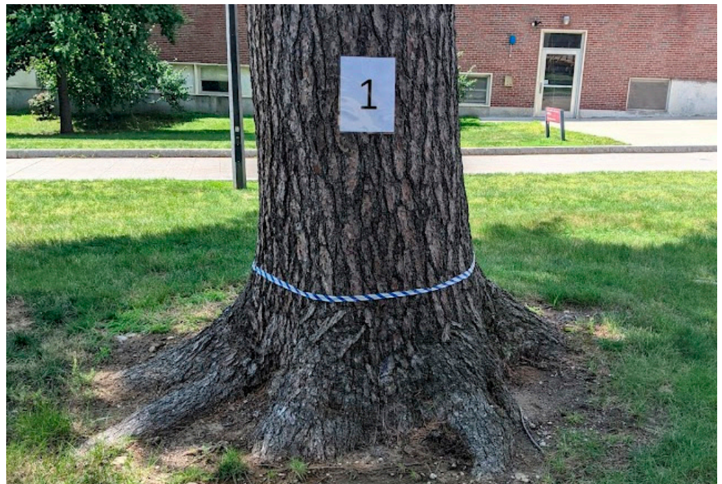
Figure 1. Lower trunk of tree 1 ( Pinus strobus ) with flagging to indicate the height at which the Resistograph drillings and tomograms were taken.
