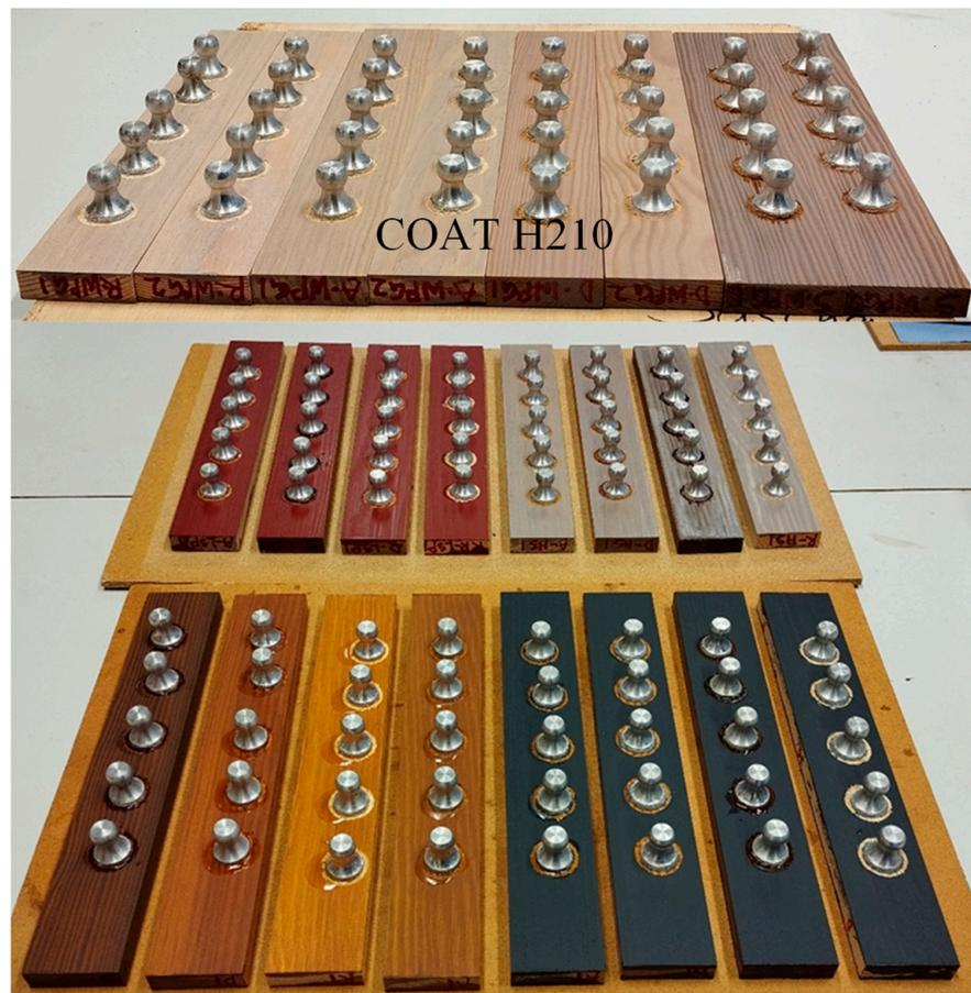
**Figure A4.** Samples of coated modified and unmodified *P. sylvestris* L. wood with glued dollies before pull-off testing.
