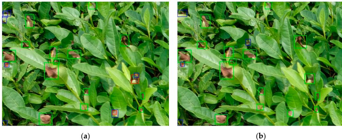
**Figure 17.** Detection of target-intensive scenarios where green boxes represent TP, blue boxes represent FN and red boxes represent FP. (a) YOLOv7's detection results. (b) Our model's detection results.
