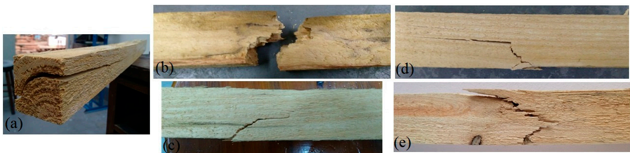
Figure 10. Horizontal shear (a), brash tension (b), cross-grain tension (c), simple tension (d), and splintering tension (e) failures observed during bending tests.
