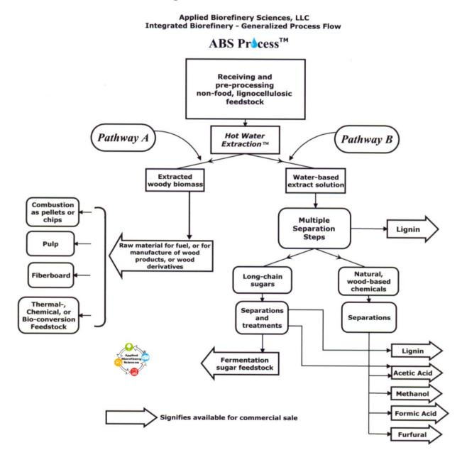
$HWE^{TM}$  in the absence of mineral acids and bases is preferred because of its ability to generate multiple high value output products without chemical input, recovery, or disposal costs. Instead of added chemicals in the cooking phase, the *ABS Process*<sup>TM</sup> relies upon an autocatalytically driven
