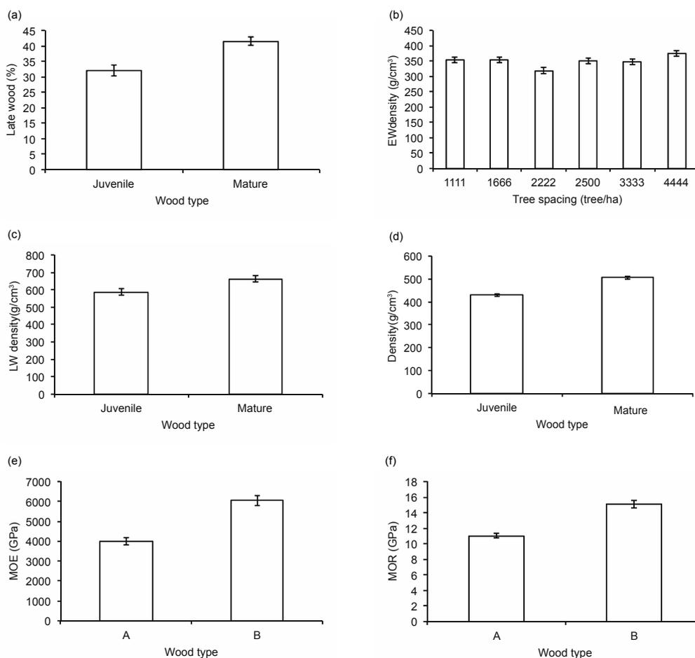
**Figure 4.** Effect of wood type on percentage of latewood (a); latewood density (c); mean wood density (d); modulus of elasticity (MOE) (e); modulus of rupture (MOR) (f); and effect of tree spacing on the earlywood density of juvenile wood (b) for jack pine 25 years following planting in Quebec, Canada. Data presented are the means ( $\pm$ SE).
