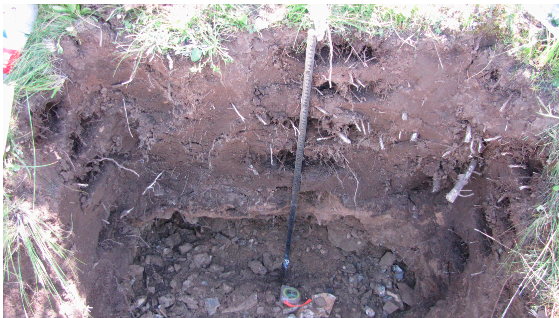
Figure 2. Plot 1 m (length) × 1.5 m (width) × 1 m (height), for collecting soil samples used for soil nitrogen density and bulk density analysis measurement.
