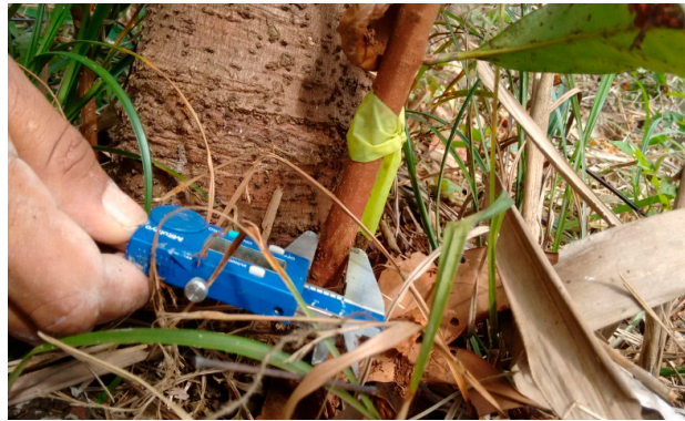
Figure A17. Measurement of shoot diameter after above ground cut at 50 cm using digital callipers in Central Amazonian commercial rosewood plantations.
