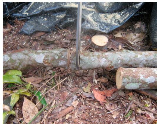
Figure A15. (Left) Collection of wood discs at 0%, 50% and 100% of the height of the stem and (Right) using chainsaws, harvesting sawdust and cutting of the trunk in sections.
