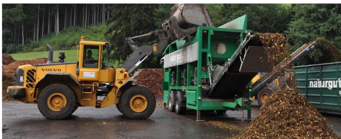
Figure 1. Mobile star screen “Multistar L3” fed by a wheeled front-end loader.
