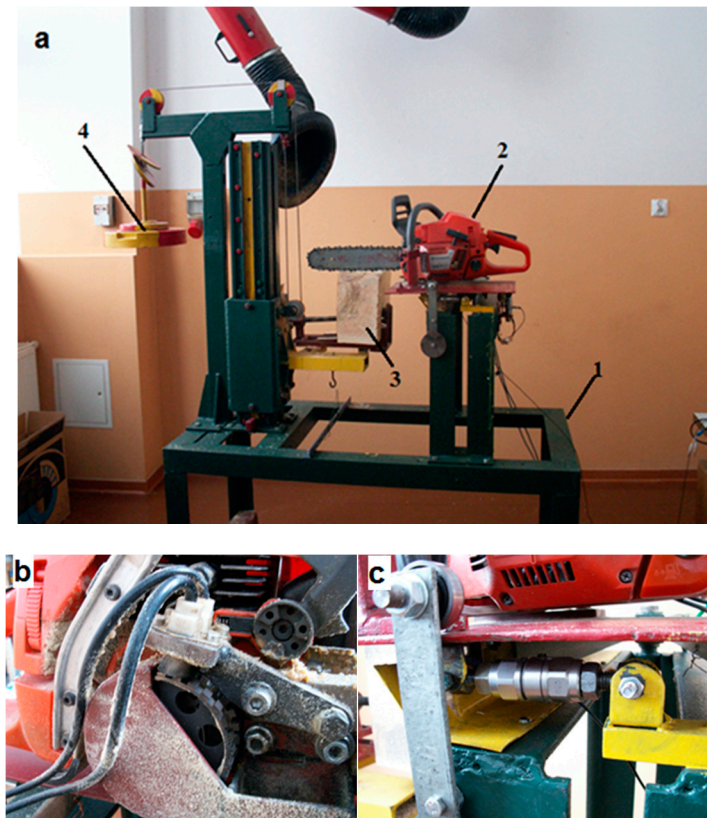
Figure 2. Real view of experimental stand for measuring chainsaw cutting parameters ((a)—general view, cutting force sensor, (b)—sensor measuring crankshaft and clutch drum rotational speed, (c)—feed force sensor, 1—base, 2—chainsaw, 3—wood sample, 4—weight).
