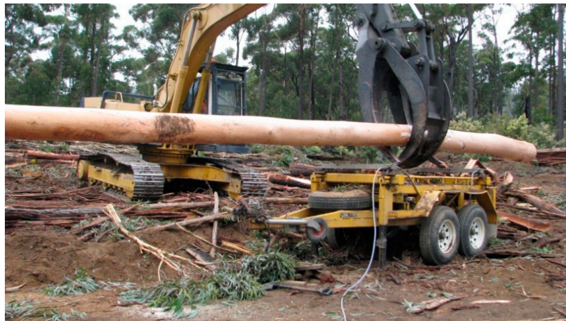
Figure 1. A debarked silvertop ash log being weighed on the biomass weighing trailer.
