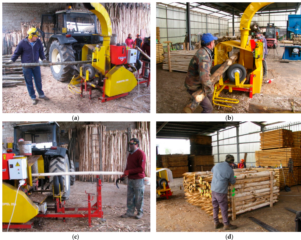
Figure 1. Typical postures assumed during post debarking at the two main work stations: loading-push (a), loading-hold (b), unloading-pull (c), and unloading-stack (d).
