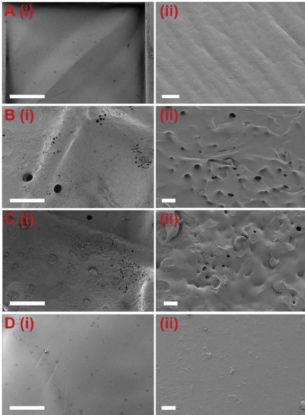
**Figure S6.** Top-view field emission scanning electron microscopy images of representative abluminal surface morphologies of the Si-covered stents with various coatings before drug release, at (A-D(i)) low and (A-D(ii)) high magnifications: (A) Si-covered stent silicone membrane surface, and (B) **Si-PU**, (C) **Si-PU<sub>5FU</sub>**, (D) **Si-PU<sub>5FU</sub>-PEVA** stent surfaces. Scale bars for A-D(i) = 500  $\mu\text{m}$ , A(ii) = 5  $\mu\text{m}$ , and B-D(ii) = 10  $\mu\text{m}$ .
