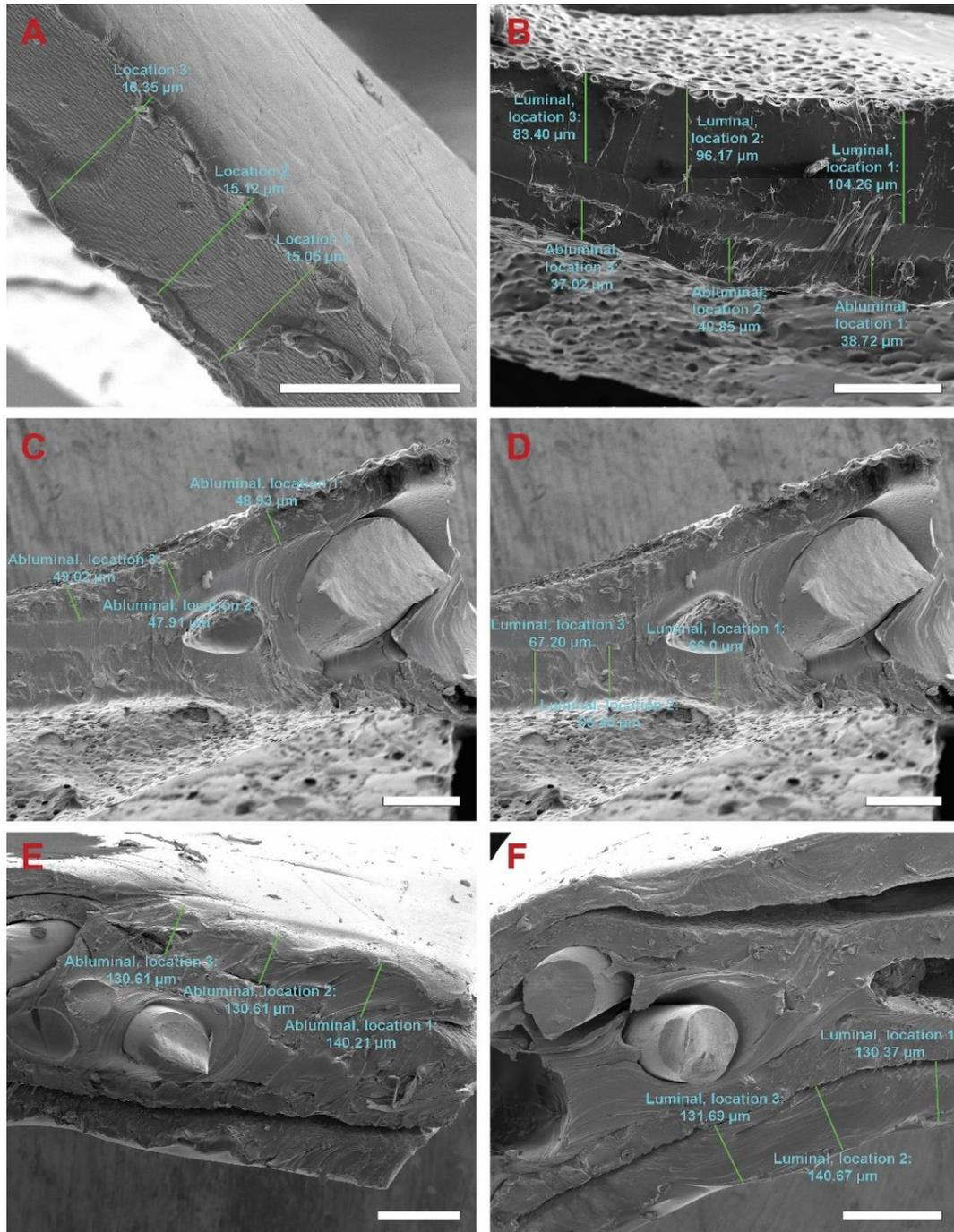
**Figure S7.** Representative cross-section scanning electron microscopy images showing coating thickness on the surface of the Si-covered stents with various coatings before drug release: (A) Si-covered stent silicone membrane cross-section, and (B) Si-PU, (C, D) abluminal and luminal Si-PU<sub>5FU</sub>, (E, F) abluminal and luminal Si-PU<sub>5FU</sub>-PEVA cross sections with measurements. Scale bars for A = 20  $\mu\text{m}$ , B-D = 100  $\mu\text{m}$ , and E-F = 200  $\mu\text{m}$ .
