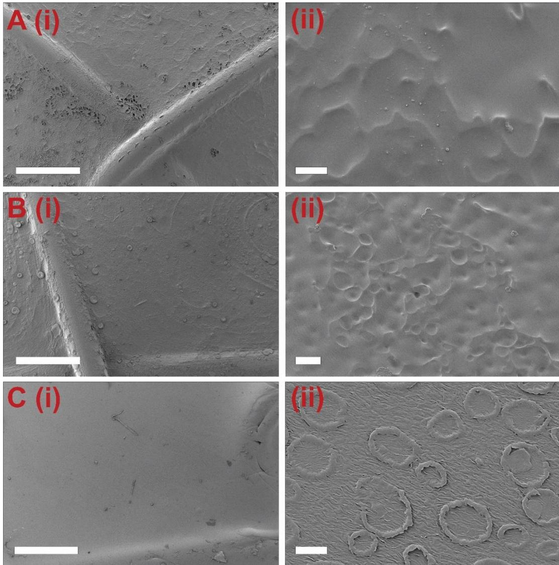
**Figure S8.** Top-view field emission scanning electron microscopy images of representative abluminal surface morphologies of the bare stents with various coatings before drug release, at (A-C(i)) low and (A-C(ii)) high magnifications: (A) **B-PU**, (B) **B-PU<sub>5FU</sub>**, and (C) **B-PU<sub>5FU</sub>-PEVA** stent surface. Scale bars for A-C(i) = 500  $\mu\text{m}$ , A(ii) = 5  $\mu\text{m}$ , B(ii) = 10  $\mu\text{m}$ , and C(ii) = 5  $\mu\text{m}$ .
