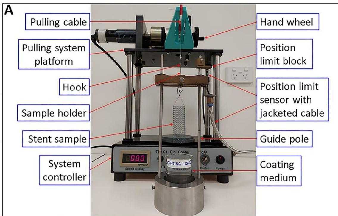
**Figure S4.** Desktop dip-coater used to prepare coated stent.
