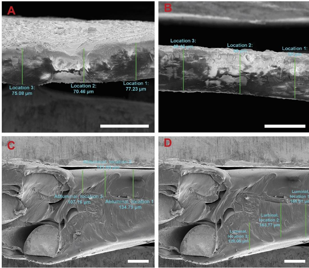
**Figure S9.** Representative cross-section scanning electron microscopy images showing coating thickness on the surface of the coated bare stent before drug release: (A) B-PU, (B) B-PU<sub>5FU</sub> (C, D) abluminal and luminal B-PU<sub>5FU</sub>-PEVA cross sections with measurements. Scale bars for A-B = 100 μm, C = 50 μm, and D = 100 μm.
