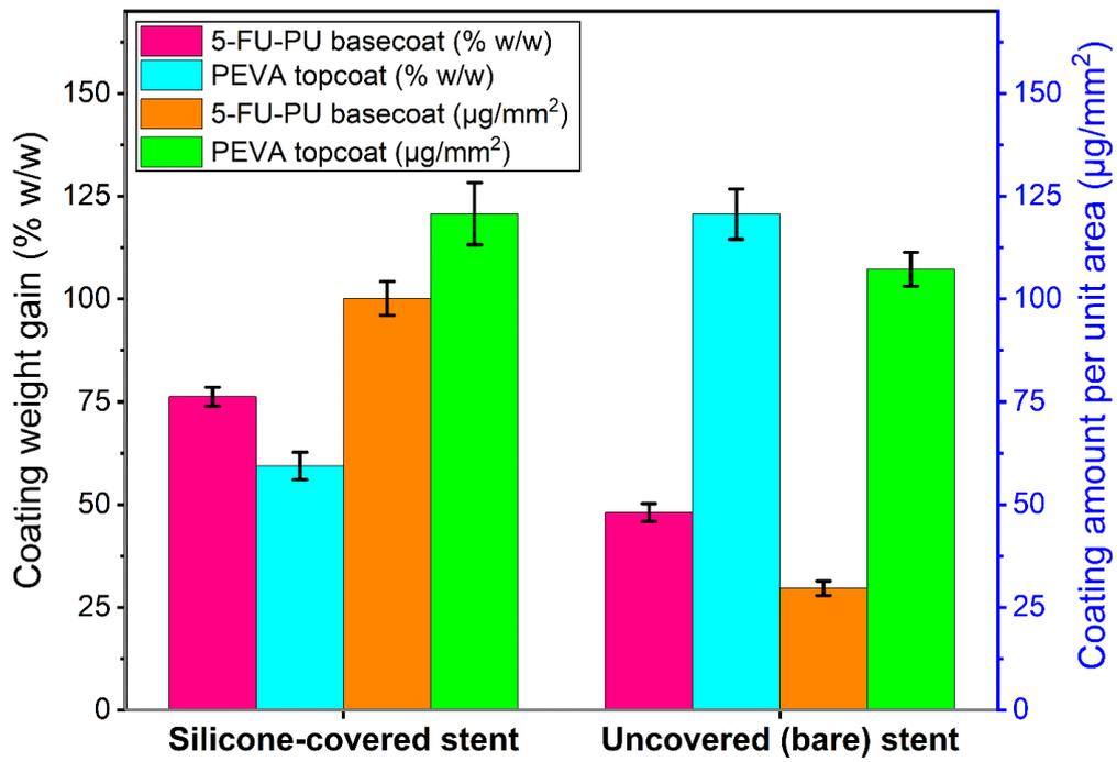
**Figure S5.** Comparison of percentage weight increase and amount of coating per unit area between the corresponding basecoat and topcoat layers of the 5FU-loaded stents. Area was calculated from both the abluminal and luminal sides of the stents. Data represent mean (n = 10) ± Standard deviation (SD).
