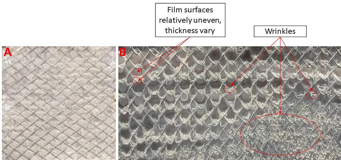
**Figure S10.** Representative luminal top-view optical images showing the PEVA topcoat surfaces of (A) Si-PU<sub>5FU</sub>-PEVA and (B) B-PU<sub>5FU</sub>-PEVA stents.
