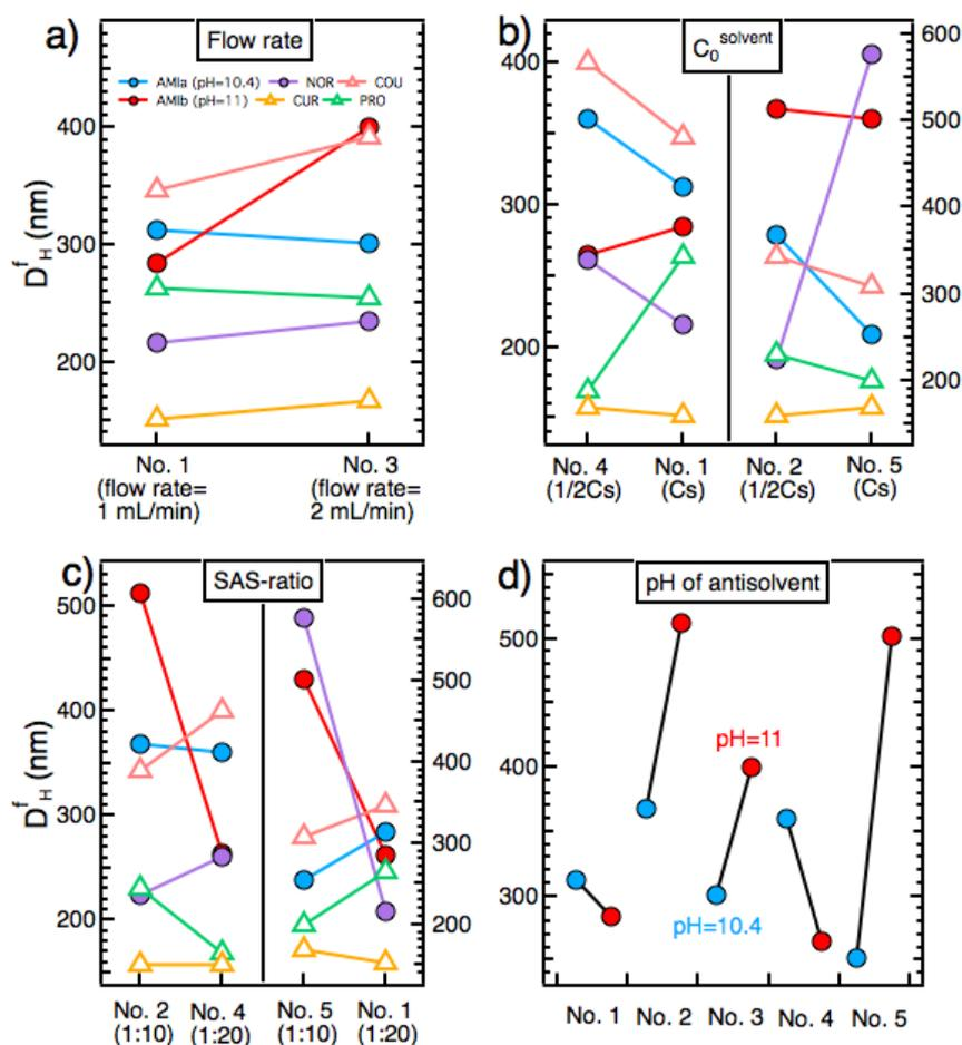
**Figure 5.** The effects of (a) flow rate, (b) compound concentration in the solvent solution  $C_0^{\text{solvent}}$ , (c) SAS-ratio (for AMIa, COU, CUR, NOR and PRO), and (d) pH of the antisolvent (for AMI particles prepared by protocols No.1–No.5; Table 2) on the final particle size  $D_H^f$ . All subfigures share the legend provided in (a).
