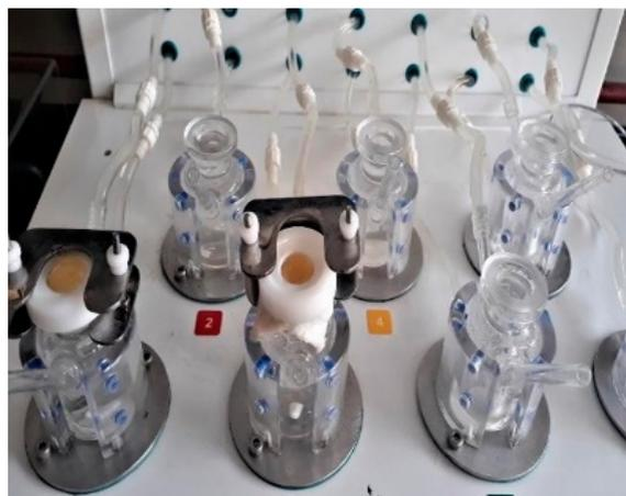
**Figure 1.** Modified vertical Franz diffusion cell apparatus.
