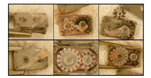
Sections through the PTFE membranes from gear devices revealed two bulbs of tissue protruding into the gear shaft holes of the device baseplate (Figure 9). Stemming from those regions, cells were present throughout the thickness of the membrane in the mid-section of the filter. The bulbs of tissue were not connected to any other internal material, suggesting that the cells had migrated through the membrane from the scleral side.
