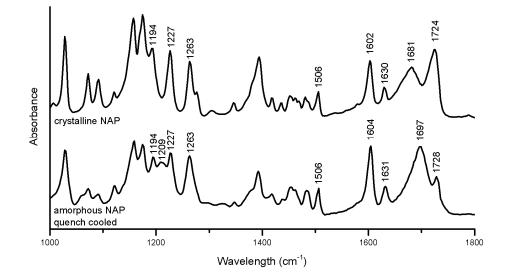
Figure 5. FTIR spectra of crystalline and amorphous NAP prepared by quench cooling.
