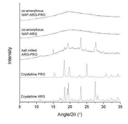
**Figure 2.** XRPD diffractograms of crystalline ARG, crystalline PRO, ball-milled ARG–PRO, co-amorphous NAP–ARG and co-amorphous NAP–ARG–PRO.
