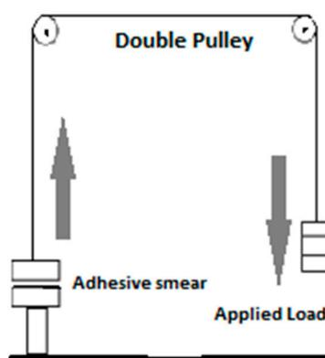
**Figure 1.** Illustration of determination of binding strength by double pulley apparatus.
