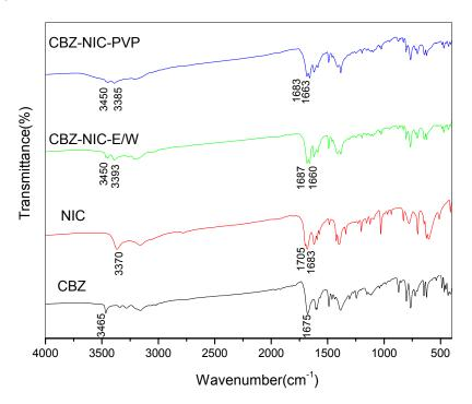
**Figure 2.** Infrared spectroscopy (IR) spectra of carbamazepine (CBZ), Nicotinamide (NIC), CBZ-NIC cocrystal screening product prepared in ethanol-water mixture (CBZ-NIC-E/W) and in polyvinyl pyrrolidone solution (CBZ-NIC-PVP).
