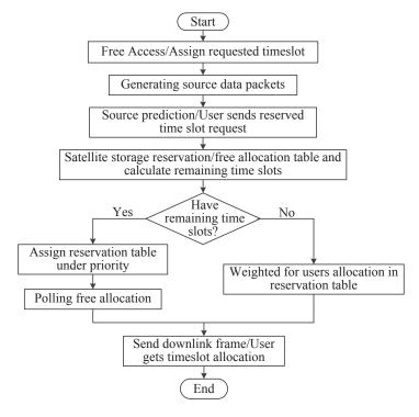
Figure 2. Flowchart of CFDAMA-GF.
