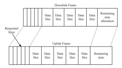
**Figure 1.** Frame structure of the combined free/demand assignment multiple access-gray forecast (CFDAMA-GF).
