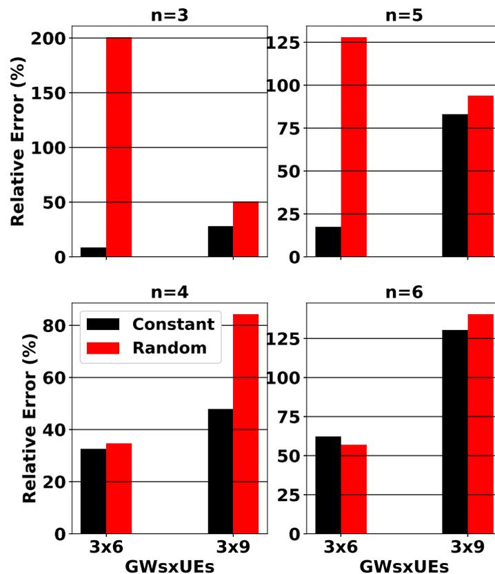
Figure 3. Average Relative Error between Exhaustive and Proposed Schemes, with Constant and Random Initial Feasible Points, for Different  $n$ th Order in  $3 \times 6$  and  $3 \times 9$  HTS Systems.
