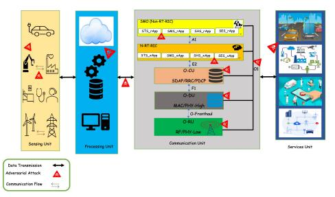
Figure 4. Attack spaces in O-RAN assisted IoT systems.
