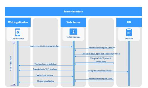
Figure 7. Sequence diagram of sensorization interface.
