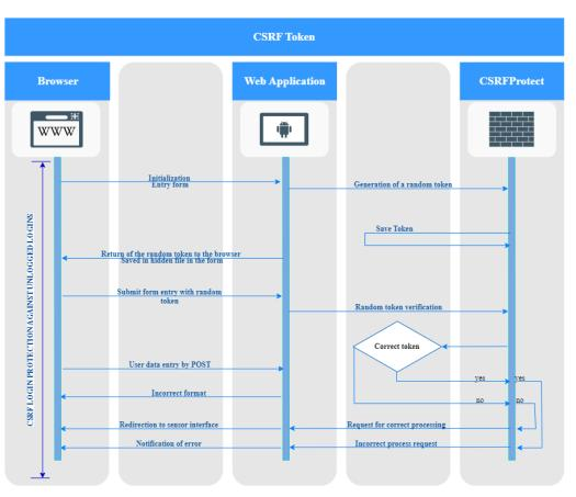
Figure 6. Sequence diagram to prevent CSRF attacks.
