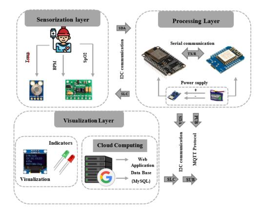
Figure 1. Architecture of the electronic vital signs measurement system.
