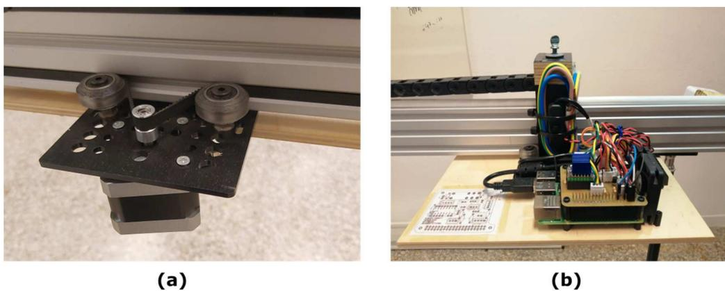
**Figure 5.** In (a), a view of the stepper motor, GT2 Timing Pulley-12T and GT2-type timing belt along with the V-Slot wheels and the carriage platform (V-slot Gantry Plate). The platform is secured to a piece of marine plywood in (b), and the TMC2209 stepper motor driver with its dedicated heatsink is shown mounted on a custom PCB Raspberry Pi shield (described in Section 2.1.3).
