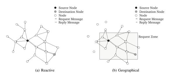
Figure 4. MANET routing algorithms.
