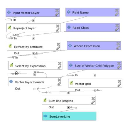
Figure 3. Processing model to compute the class-wise length of features with "name" attributes.
