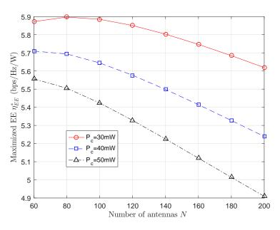
Figure 6. The maximized energy efficient versus the number of antennas.
