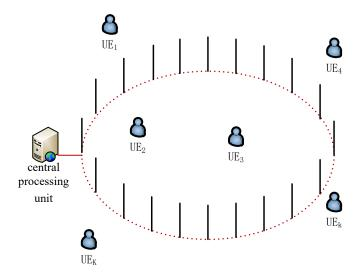
**Figure 1.** Massive multiple-input multiple-output (MIMO) system with circularly distributed antennas; *K* user equipments (UEs) simultaneously transmit signal to the base station (BS) with *N* antennas located on a circle with radius *r*.
