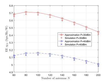
Figure 2. The energy efficiency (EE) versus the number of antennas.
