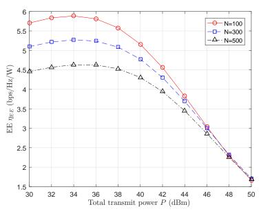
Figure 4. The energy efficiency versus the total transmit power.
