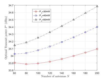
Figure 5. The optimal total transmit power versus the number of antennas.
