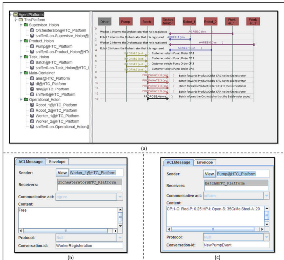
Figure 10. (a) Workcell Setup and Batch Order Building; (b) ACL Message holds the Worker Registration; (c) ACL Message holds the product details.
