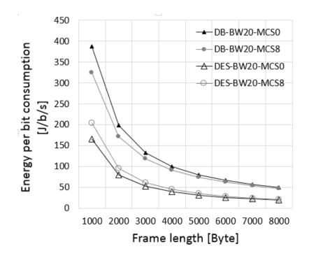
Figure 7. Energy consumption over different frame lengths.
