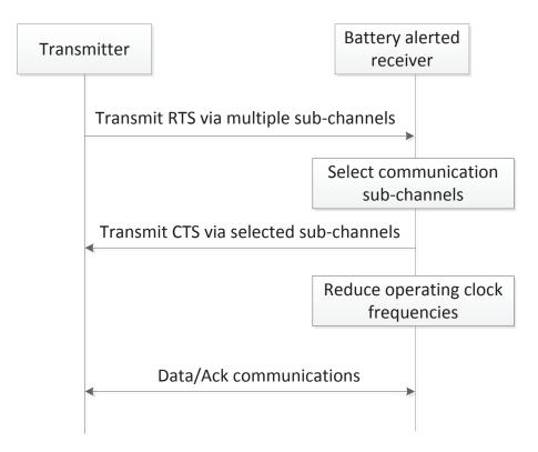
Figure 3. Flowchart for dynamic energy saving operation.
