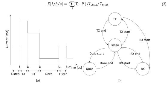
**Figure 5.** Energy consumption model: (**a**) current consumption for power states; and (**b**) power state flow control; TX: transmission; RX: reception.
