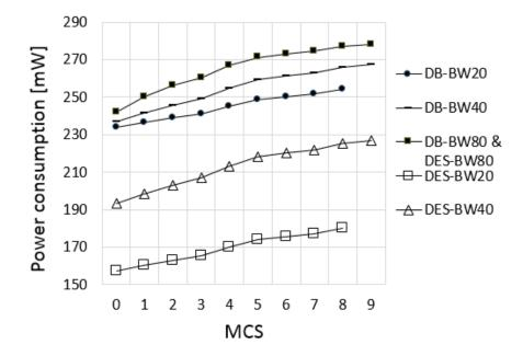
**Figure 6.** Energy consumption over various parameters: MCS, bandwidth, and operating scheme in the active mode.
