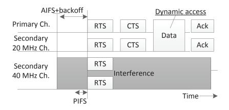
**Figure 1.** Dynamic bandwidth allocation mechanism; CTS: clear to send; RTS: request to send; Ack: acknowledgment; PIFS: point coordination function.
