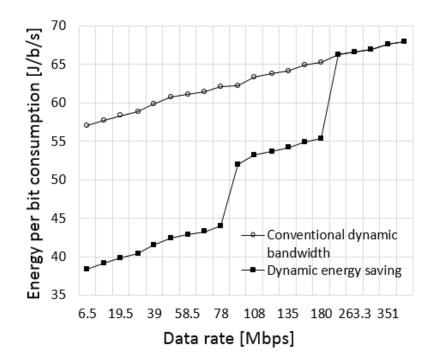
Figure 8. Energy consumption over data rates when using the link adaptation scheme.
