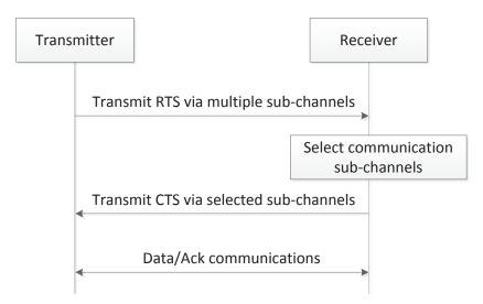
Figure 2. Flowchart for dynamic bandwidth allocation.
