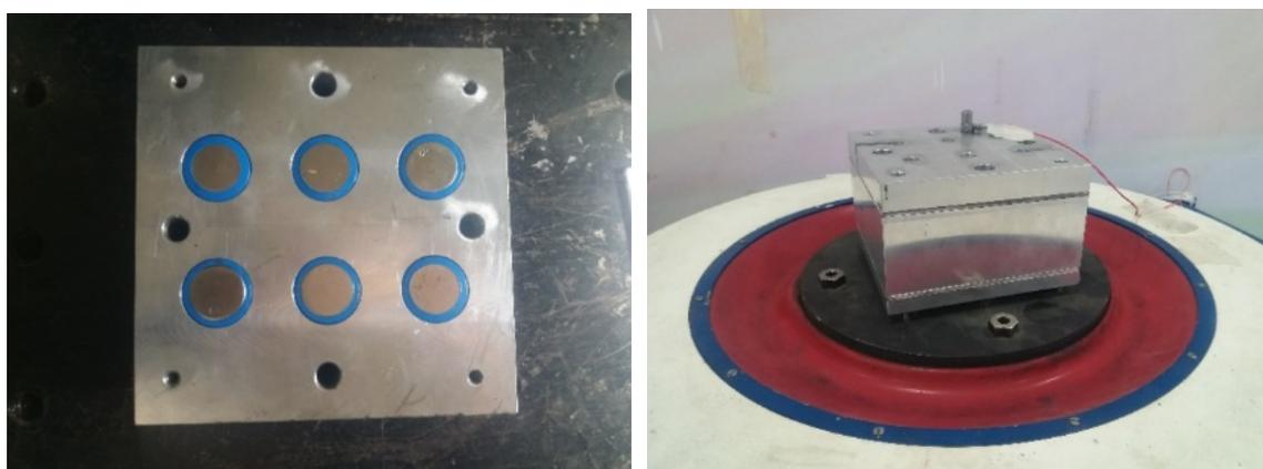
Figure 1. Vibration test fixture and setup.
