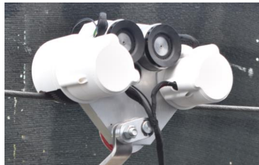
Figure 24. Trolley traction structure with 3D-printed cover.
