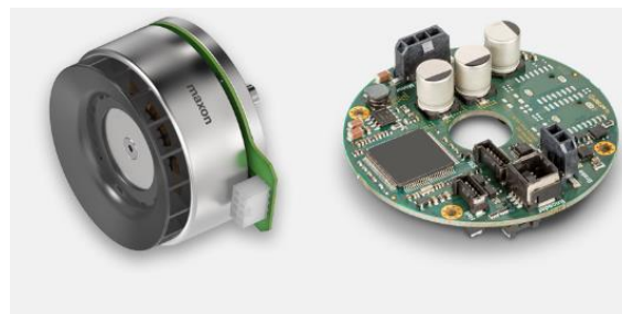
Figure 21. Chosen motor (left) and the inverter (right).
