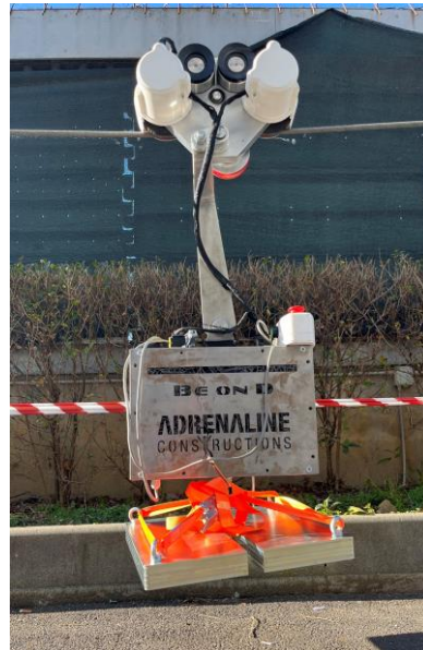
Figure 33. Electric trolley with 55 kg payload.
