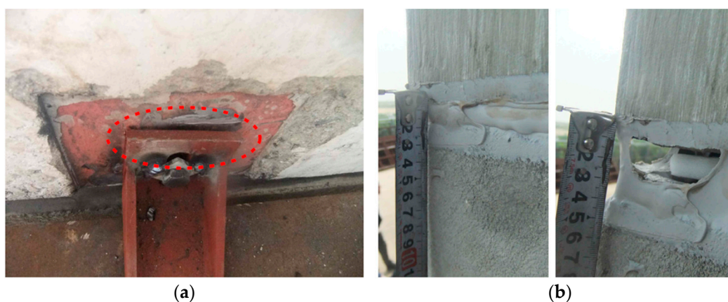
Figure 8. Results of second relative story displacement test: (a) Fastener damage; (b) Horizontal joint damage.
