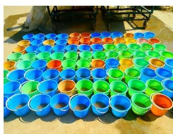
**Figure 5.** Runoff and sediment were collected at intervals of two min after runoff was produced. Water and sediment were separated by the static precipitation method.
