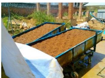
**Figure 3.** Simulated slopes under 5 degrees and 10 degrees (the air-dried tested soil was loaded into the soil-bins according to layer. The size of the soil-bin was 2.0 m × 1.0 m × 0.5 m, and its slope was adjustable. There was a captation for collecting runoff and sediment at the bottom of the soil-bin.).
