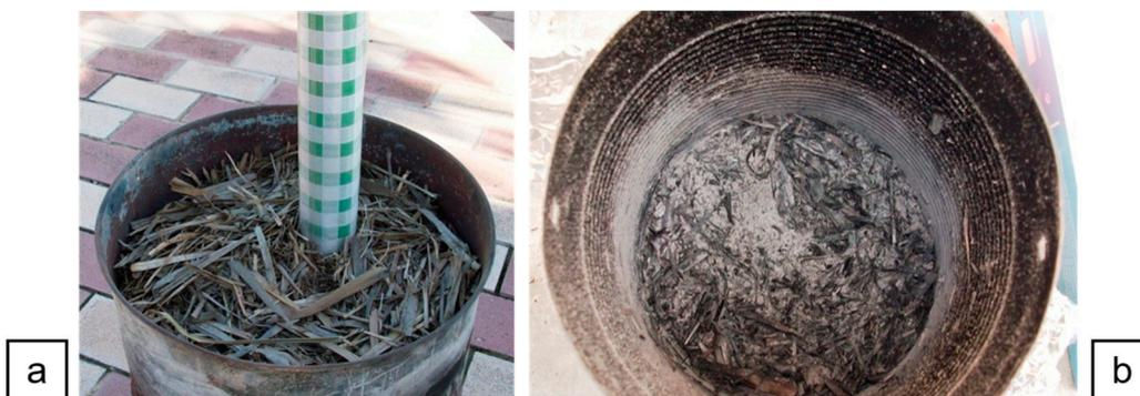
**Figure 9.** Autocombustion container: (a) *Arundo donax* leaves and sheath leaves before ignition; (b) remaining ashes after autocombustion.
