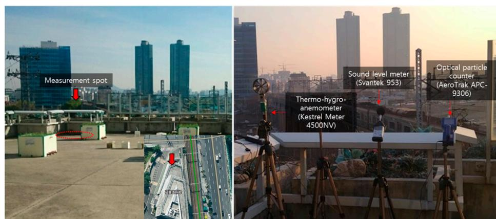
**Figure 2.** Measurement spot (left) and the recording set-up (right) on the site.
