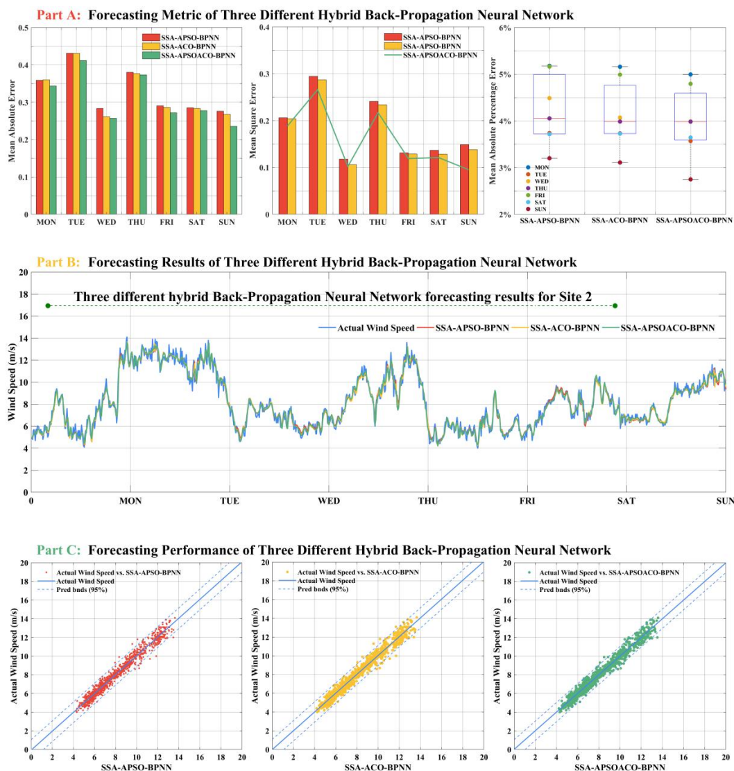
Figure 5. The results of three different BPNN forecasting models in site 1.
