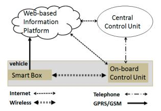
Figure 1. Conceptual representation of a smart logistics system (SLS).
